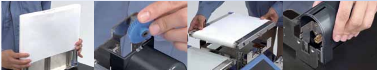
Replacing a belt
